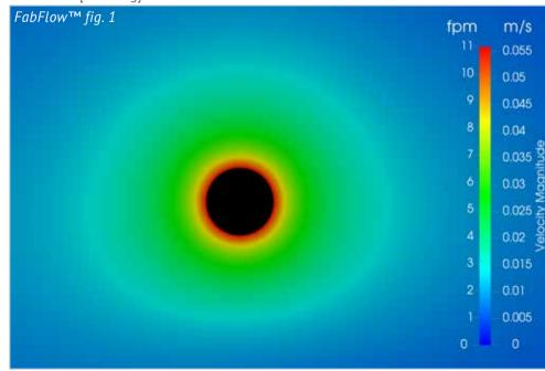
Examples of CFD simulations with FabFlow™ at 3 m [≈10 ft] above floor level. The occupied zone is indicated by the black line 1.8 m [≈6 ft] above floor level. Cold air exits the duct and moves downward due to thermodynamic forces. The gentle air diffusion accumulates and develops a uniform airflow as temperature difference increases. The airflow gains more momentum and the velocity increases with the distance from the duct.
