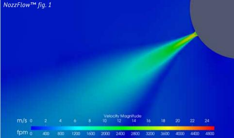
The flow is accelerated due to the conical shape of the nozzle. The acceleration rate depends on the static pressure inside the duct. The characteristics of NozzFlow™ makes it possible to precisely direct the air exactly where it is required.
