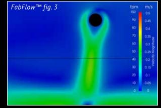
Air permeability 200 m<sup>3</sup>/h/m<sup>2</sup> [10 CFM/ft<sup>2</sup>] at 120 Pa [ $\approx$ 0.5 iwg], cooling with  $\Delta$ T of -5 K. Microperforation enables a higher cooling capacity while keeping the occupied zone draft-free.
