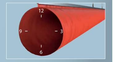
When working with round profiles, we use clock positions to determine the placement of the appropriate flow model(s). We always determine clock positions with the airflow coming from our back. Often permeable fabrics or microperforations are used in order to prevent dust from settling inside or onto the duct.
