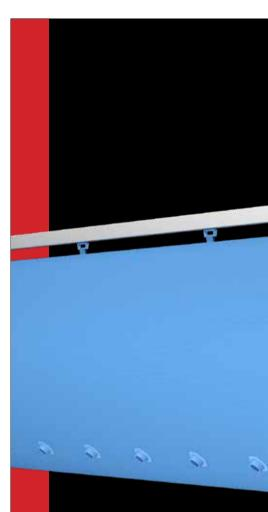
Example of Typical Application: Spot cooling at 7m [23 ft],  $\Delta T$  of -7 K and 120 Pa [ $\approx$ 0.5 iwg] static pressure. The air is delivered exactly where it is required – marked by the highlighted box.
