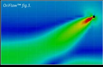
Example: Air pattern in <u>heating</u> with  $\Delta T$  of +6 K and 120 Pa [ $\approx 0.5$  iwg] static pressure in a theoretical large space.
