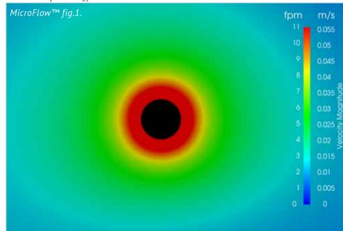
Examples of CFD simulations with MicroFlow™ at 3 m [≈10 ft] above floor level. The occupied zone is indicated by the black line 1,8 m [≈6 ft] above floor level. When the cold air exits the duct, it moves downward due to thermodynamic forces and merges into a uniform airflow that gains momentum as it moves away from the duct.
