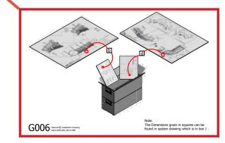
Once produced, the air dispersion system undergoes final inspection, and a full overview of all order items listed by box number is created. This overview is always added as a checklist in Box no. 1 along with relevant documents like installation guide, laundry and maintenance manuals and the spec drawings.
