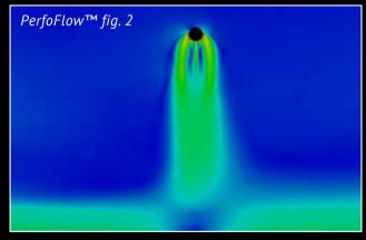
Air diffusion with perforation of  $@ 10 \text{ mm} [\approx 0.4 \text{ in}]$ holes located at 180° over 6 o'clock position. Cooling at  $\Delta T$  of -6 K.
