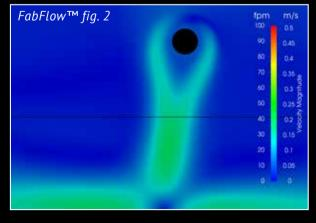
Air permeability 200 m<sup>3</sup>/h/m<sup>2</sup> [10 CFM/ft<sup>2</sup>] at 120 Pa [ $\approx$ 0.5 iwg], cooling with  $\Delta$ T of -3 K. Increased cooling capacity and draft still avoided.
