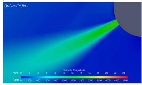
With OriFlow<sup>™</sup>, the air exits at discharge velocity, which decreases with traveled distance from the duct and depends on the static pressure inside the duct. With a properly designed air dispersion system, OriFlow<sup>™</sup> is strong enough to ensure heating in medium to high installation projects. 1000000
