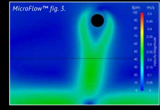
Air permeability 200 m<sup>3</sup>/h/m<sup>2</sup> [10 CFM/ft<sup>2</sup>] at 120 Pa [ $\approx$ 0.5 iwg], cooling with  $\Delta$ T of -5 K. Microperforation enables a higher cooling capacity while keeping the occupied zone draft-free.
