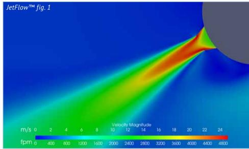
The flow is accelerated due to the conical shape of the jet. The acceleration rate depends on the size of the jet and the static pressure inside the duct. As the discharge coefficient is very close to 1.0, it is possible for the supply air to penetrate the space with high precision at very long throws.
