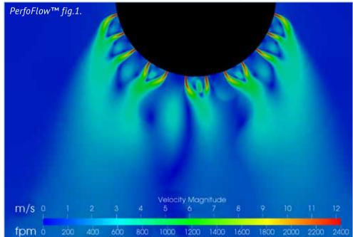
Air discharge through PerfoFlow<sup>™</sup> perforation at 120 Pa [≈0.5 iwg].
