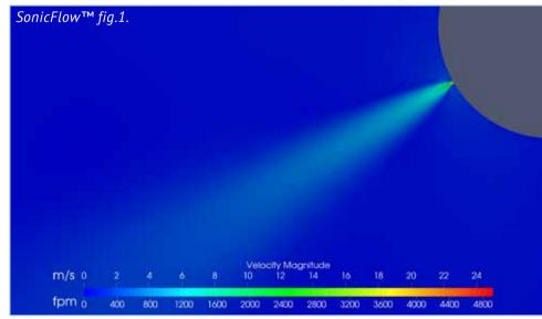
With SonicFlow<sup>™</sup>, the air exits at discharge velocity, which decreases with traveled distance from the duct and depends on the static pressure inside the duct. Fig. 2 shows an example of a CFD simulation with SonicFlow<sup>™</sup> at 3 m *[≈10 ft] above floor level. The occupied* zone is indicated by the black line 1.8 m [≈6 ft] above floor level. Figs. 3 and 4 shows the differences in airflow patterns between cooling and heating in scenarios with identical parameters.
