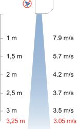
According to standard NSF-37-2012, in service windows must be an air jet at 3,05m/s of 200mm width at 1/3 of the window counter top.
