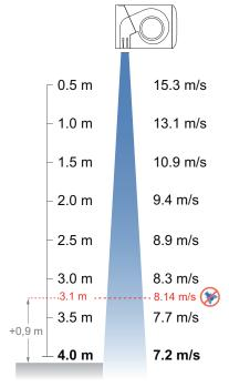
According to standard NSF-37-2012, the maximum installation height is the speed profile point at 8,14m/s plus 0,9m. So FLY KXL can be used until 3,1m+0,9m=4,0m.
