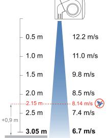
According to standard NSF-37-2012, the maximum installation height is the speed profile point at 8,14m/s plus 0,9m. So FLY KL can be used until 2,15m+0,9m=3,05m.
