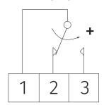
Humidification Dehumidification Closing contact between terminals 1 and 2 Closing contact between terminals 1 and 3
