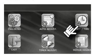
• To set the date and time on the control panel, go to the User menu by pressing (see para. 5) and then press **DATE, TIME**.
