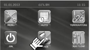
• To activate the timer, press **TIMER** in the control panel Main menu.
