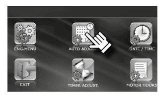
• To set up the **AUTO** mode, press the button to enter the User menu, see para. 5, and press **AUTO ADJUST**
