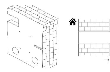
**4.** Fill the spaces between the air ducts and the wall with a mounting foam through the specially designed holes in the mounting template. Wait till a mounting foam hardens then take off the mounting template and remove the foam excess. Cut off the protruding air duct parts to be flush with the wall surface.
