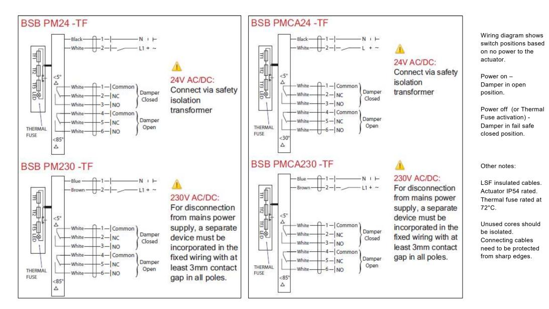
For damper closed indication use terminals 1 & 2 For damper open indication use terminals 4 & 6 Terminals 1 & 4 can be linked where required as an option.
