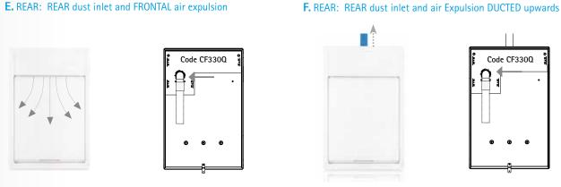
For rear installations, both with the FRONTAL air expulsion (fig. E) and with the UP air expulsion (Fig. F), must be used the rear installation kit for wall-mounted QB in thermoplastic material Cod. CF330Q
