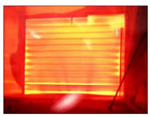
Damper blades glowing during a vertical fire test
