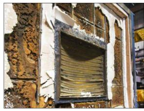
Remains of a drywall partition after a fire test
