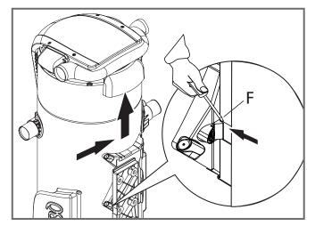
**6** - To unhook the central power unit from the support, press the lock hook with the help of a screw driver (F). Slide the central power unit to the left and lift it.
