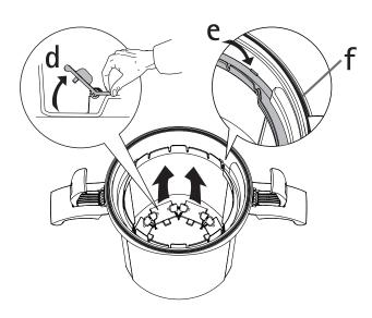
${f 2}$  - Insert the CLEAN BAG in the dust container ensuring that the blue disc (printed on the bottom of the bag) is placed at the centre of the container.
