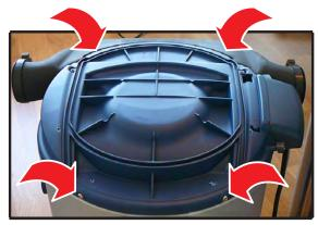
$\boldsymbol{6}$  – unhook the fastening spacers, disconnect the AVT card power supply cable and replace it.
