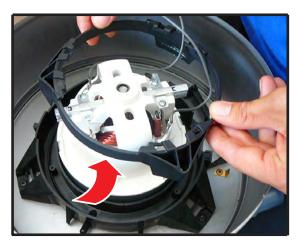
$\boldsymbol{5}$  – insert the fixing ring so that the centring supports enter the appropriate joints.
