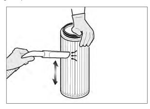
**2** - After an initial brief cleaning, wash the filter cartridge with a jet of water that is not too strong and remove the dust that penetrated between the walls.
