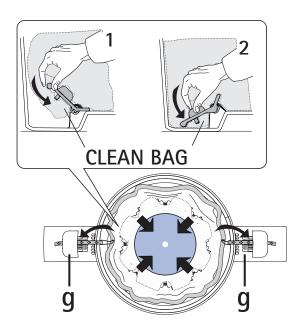
${f 3}$  - Fold the upper part of the bag inside the bag tensioner ring (k). The CLEAN BAG must adhere to the internal walls of the dust container.
