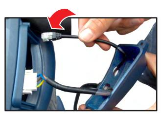
${f 3}$  Insert the new wireless cable in the free hole and connect it to the dedicated LM2 plug inlet.
