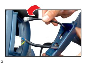
Insert the new wireless cable and connect it to the dedicated LM2 plug inlet.
