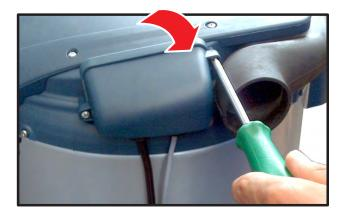
**1** Open the power unit's electric connection casing.
