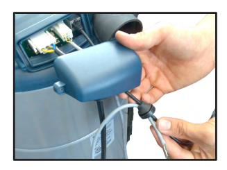
Insert the endless end into the cable gland where the wireless cable was already inserted.
