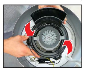
**5** - extract the motor, remove the 2 seal gaskets and replace it.
