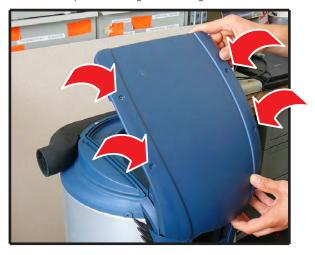
**3** - unscrew the 2 upper screws and the two screws in front of the front casing.
