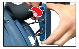
Insert the cable gland in the specific hole and close the casing.
