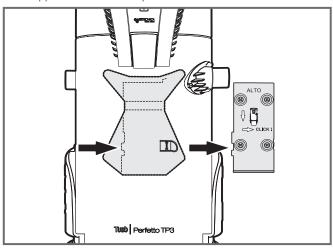
**5** -The lock hook must release with a CLICK; use a screwdriver for leverage if necessary (see figure 6, letter F).
