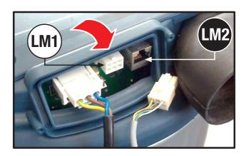
**2** Disconnect the micro line connector LM1 and remove its cable with the cable gland.
