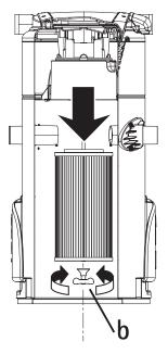
**3** - Insert a new cartridge and tighten the knob completely (b). The alignment system guarantees perfect filter cartridge fastening.
