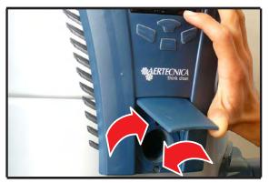
1 - Open the casing, unscrewing the two screws on the sides. Disconnect 5 - remove the front casing after disconnecting the connector and the rubber tubes.
