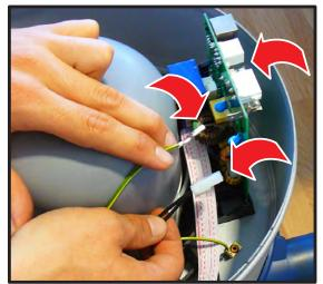
**3** - unscrew the 3 motor fixing screws.
