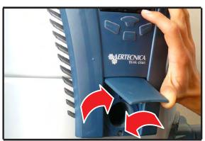
$\boldsymbol{4}\,$  – remove the front casing after disconnecting the connector and the rubber tubes
