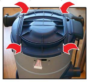
$\boldsymbol{2}$  – disconnect the motor-card connector and remove the power card.
