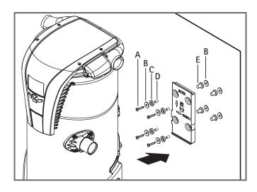
**3**- Stand with the central power unit in front of the bracket and use a downward movement to hook the central power unit support to the bracket slide.
