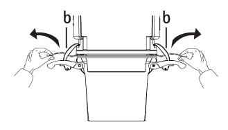
**3** - Unhook the container from the support by opening the levers (c) sideways and put it on the ground.
