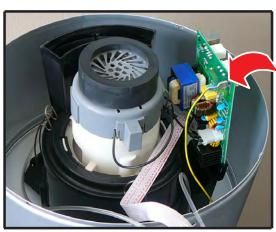
**3** - open the 3 hooks that fasten the motor.
