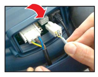
Reinsert the LM1 micro line connector into its dedicated inlet and insert the other cable end into the hole together with the one from the LM2 line.
