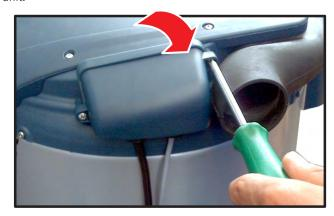
Open the power unit's electric connection casing.
