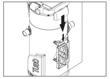
**4**- With a simple left to right movement, slide the central power unit support to the end stop.
