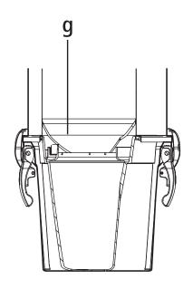
**3** - Insert a new cartridge and tighten the knob completely (b). The alignment system guarantees perfect filter cartridge fastening.
