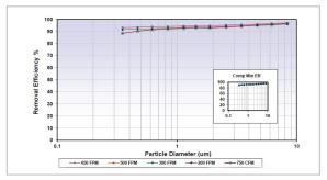
Particle Size Removal Efficiency
