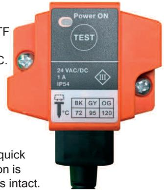
For safety reasons the TF is designed to operate only once upon reaching the activation temperature. Cutting the cable to the TF with the power on will trip an electrical fuse within the actuator, rendering it inoperable.
