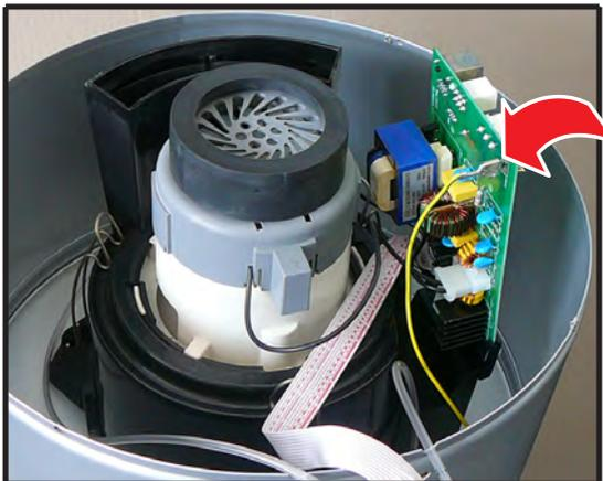
3 - open the 3 hooks that fasten the motor.
