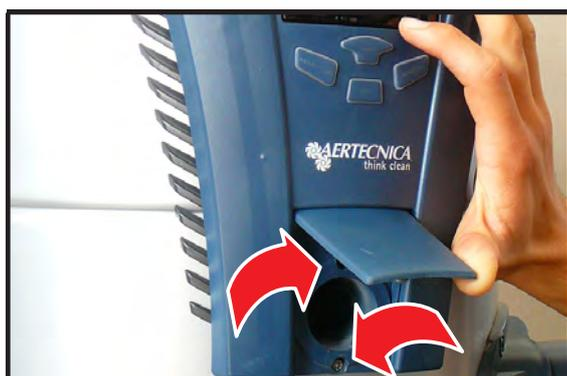
4 - remove the front casing after disconnecting the connector and the rubber tubes
