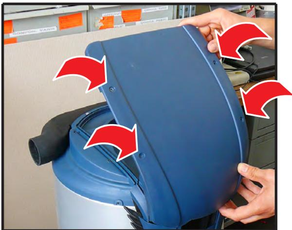
5 - open the motor compartment unscrewing the 4 screws.
