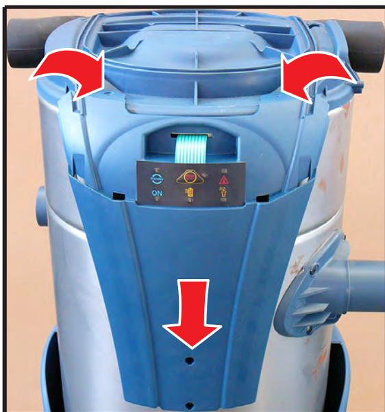
6 - unhook the fastening spacers, disconnect the AVT card power supply cable and replace it.
