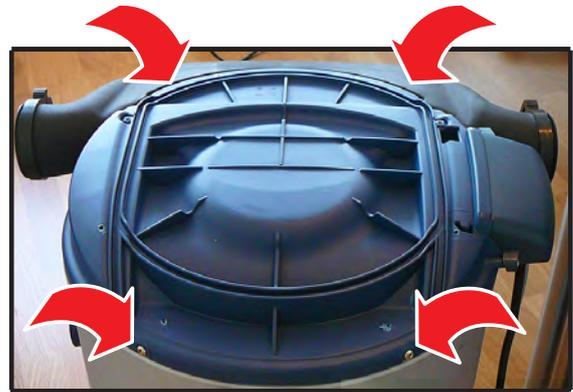
3 - unscrew the 2 upper screws and the two screws in front of the front casing.
