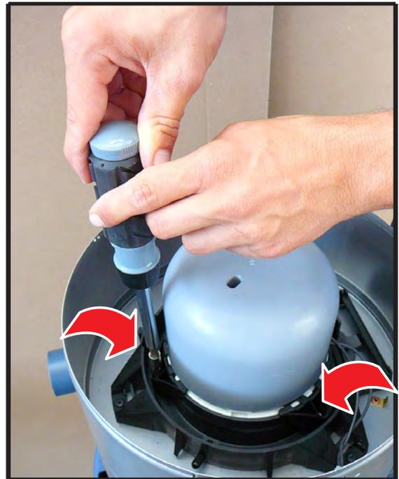
4 - remove the motor fixing ring and replace the motor.
