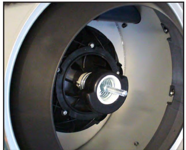
3 - Check with a test lasting a few seconds that the beater and spring rotate regularly and correctly around the central pivot.
