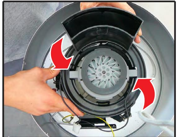
5 - extract the motor, remove the 2 seal gaskets and replace it.
