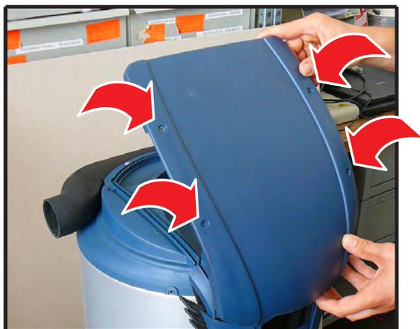
2 - unscrew the 2 upper screws on the front casing.
